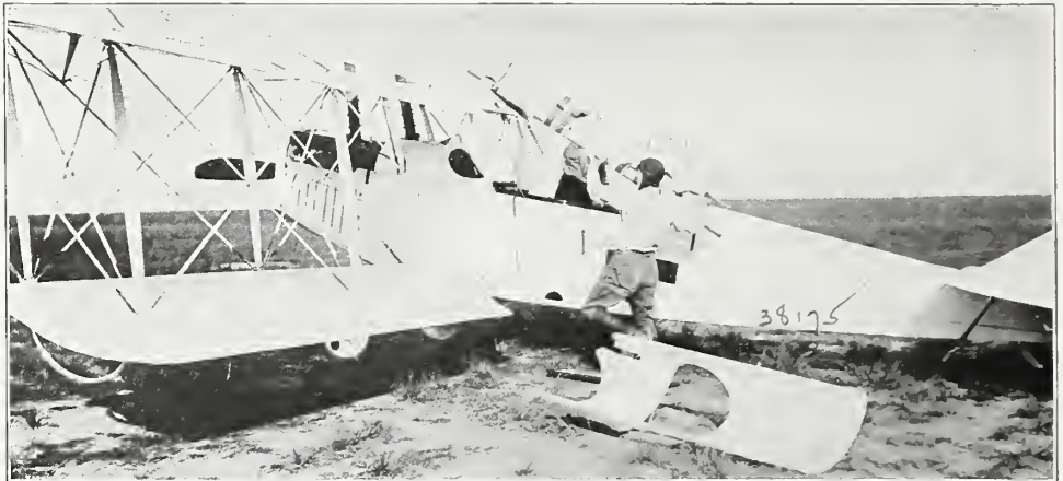
FIG. 143.—JN-4H airplane ambulance. Top removed from fuselage; litter being removed.
